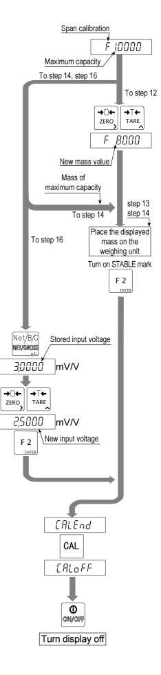
Press and hold the ON/OFF key and press the ESC key.
