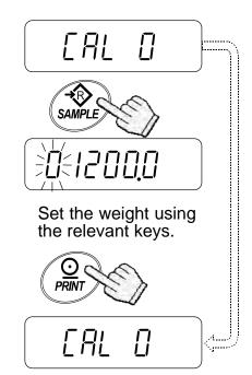
5. At step 3, pressing the PRINT key weighs the zero-point value. Do not touch the pan during weighing.
