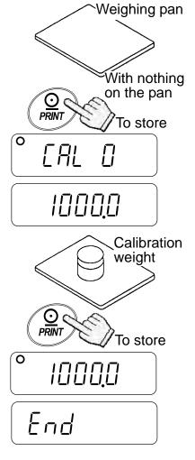
6. Place the calibration weight with the same value as displayed on the pan. Press the PRINT key to weigh it. Do not touch the pan during weighing.
