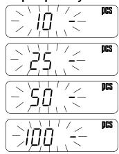
When sample weight is light and the counting error could become large, the balance will prompt you to use a larger number of samples. Place the displayed number of samples on the pan and press the PRINT key to store the unit weight.
